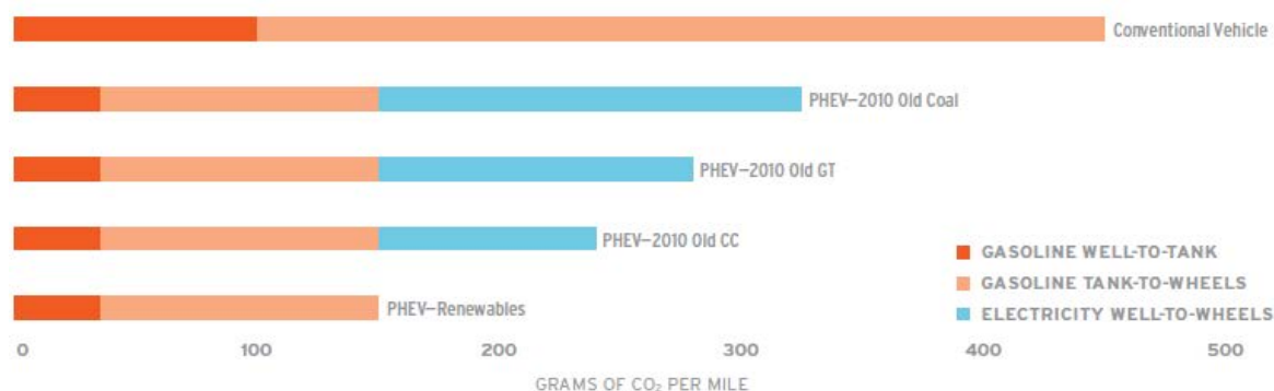
Figure 1-5: Well-to-wheel scenarios for electric vehicles
